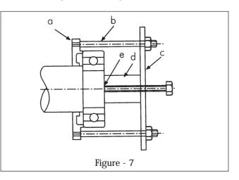
and the pressure should be uniformly distributed, parallel with the shaft and at right angles to the bearings.
