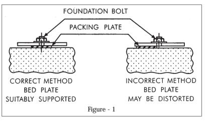
on a base slide rail which in turn is placed on the foundation with steel packing plates (Shims) in between them. The shims are evenly placed 25 to 30 cm apart and are situated close to and on each side of every foundation bolt as shown in figure to protect the base plate from suffering distortion by providing mechanical support to it.
